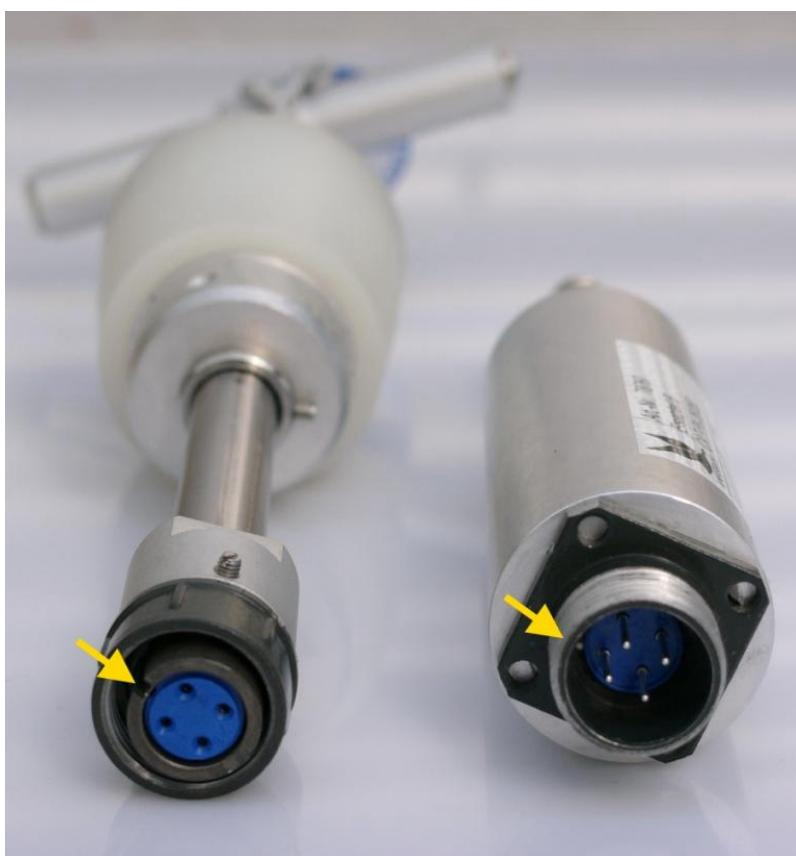
**Figure 13: Connection between the upper part and the ozone part: fitting nose must match (see arrows)**
